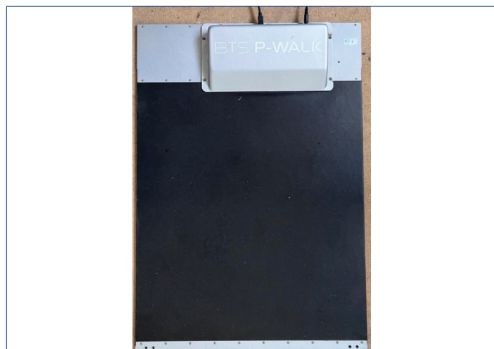
[Table/Fig-1]: BTS P-WALK foot pad, used for foot pressure analysis and percentage surface area of foot calculation in this study.
