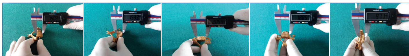
[Table/Fig-2]: Measurement of Anteroposterior Diameter-Superior (APD-S). [Table/Fig-3]: Measurement of Anteroposterior Diameter-Inferior (APD-I). [Table/Fig-4]: Measurement of Transverse Diameter-Superior (TD-S). [Table/Fig-5]: Measurement of Transverse Diameter-Inferior (TD-I). [Table/Fig-6]: Measurement of Height Anterior (HA). (Images from left to right)
