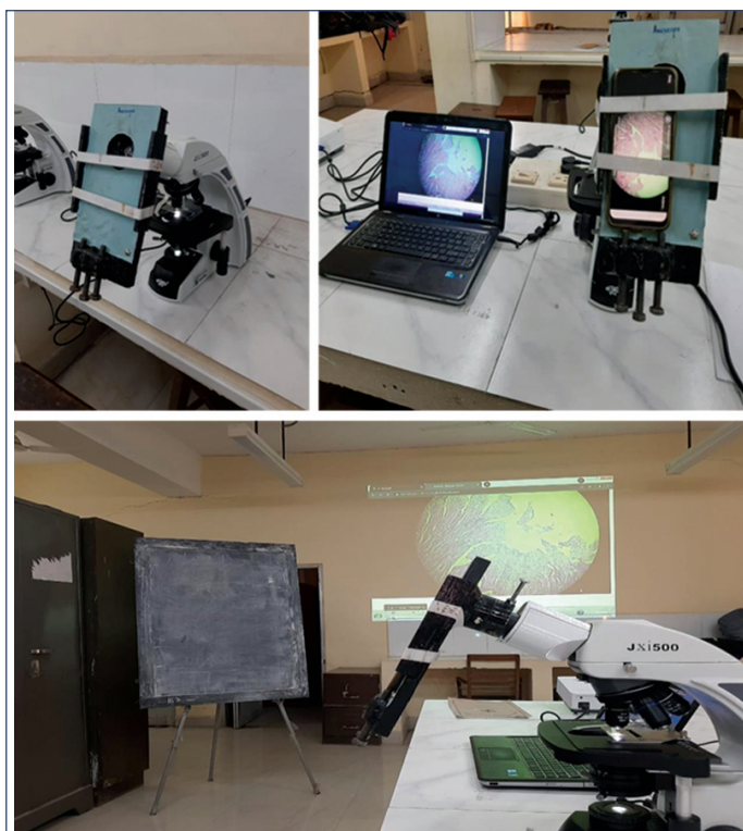
[Table/Fig-1]: Device and the whole setup for histology classes.
